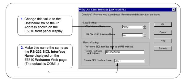
4 Do Not Delete the LAN Client Interface. When the VISA LAN Client is configured, the LAN Client is also automatically configured in the background. Thus, when VISA LAN Client configuration completes, two configured interfaces are displayed on the IO Config main screen. See the following figure for a typical display. Do NOT remove the LAN Client or VISA LAN Client interface, as the application will not run if either interface is removed
