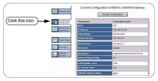
3 Display the Modify Configuration Page. From the Current Configuration of E5810 LAN/GPIB Gateway page, click the Modify Configuration button to display the Password dialog box.
