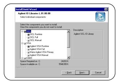
b Select the components you want to install and clear the components you do not want to install. Then, click <u>Next></u> to display the <u>Current Settings</u> dialog box. This box shows the (default) paths in which VISA and SICL will be installed and the components that will be installed.
