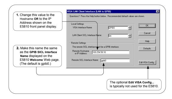
4 Do Not Delete the LAN Client Interface. When the VISA LAN Client is configured, the LAN Client is also automatically configured in the background. Thus, when VISA LAN Client configuration completes, two configured interfaces are displayed on the IO Config main screen. See the following figure for a typical display. Do NOT remove the LAN Client or VISA LAN Client interface, as the application will not run if either interface is removed.
