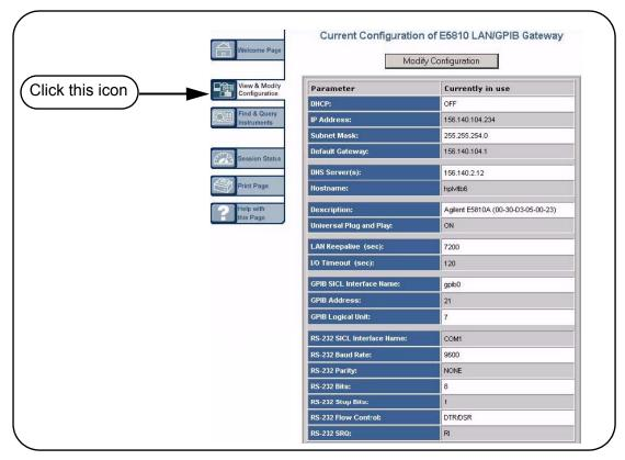
3 Display the Modify Configuration Page. From the Current Configuration of E5810 LAN/GPIB Gateway page, click the Modify Configuration button to display the Password dialog box.
