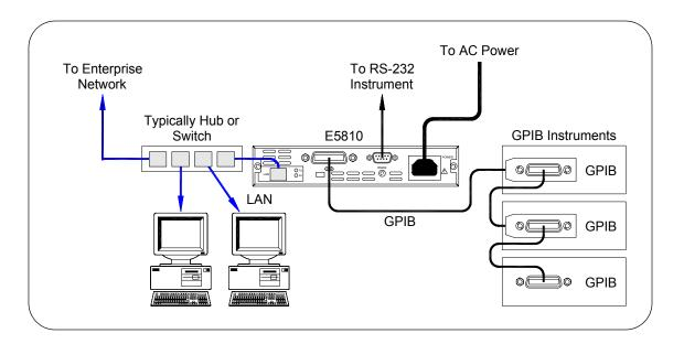
After connecting the E5810 to the Enterprise network, plug the E5810 AC power cord into an AC outlet and observe the power-on sequence. When the power-on sequence is complete, the assigned IP address of the E5810 is displayed on the second line of the front panel display. A typical display follows. See *Chapter 1 - E5810 Description* for power-on sequences.
